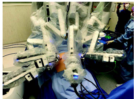
Figure 2 - Docked XI system for robotic redo hiatal hernia surgery
