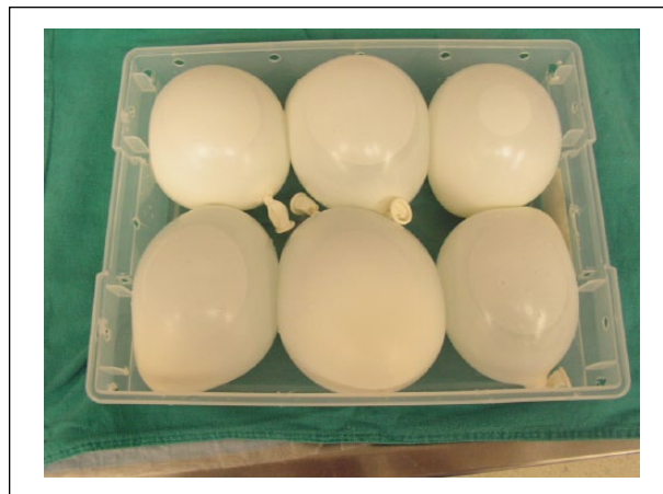
Figure 3. Water filled balloons placed in plastic container. Note holes along edges of container.
