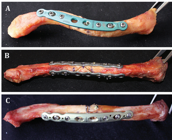
Figure 1. (A) Right clavicle plated superiorly by use of an 8-hole titanium precontoured clavicle plate ( 98 \times 11 \times 3.3 mm) fixed with a total of six 3.5-mm cortex screws placed bicortically and a 2.3-mm interfragmentary (IF) screw for the inferior butterfly fragment. (B) Right clavicle dual plated with a 7-hole titanium 2.7-mm plate ( 85 \times 11 \times 1.6 mm) positioned superiorly and another 7-hole 2.7-mm plate positioned anteroinferiorly. A total of four 2.7-mm cortex screws placed bicortically were used for each plate (8 screws total) along with a 2.3-mm IF screw for the inferior butterfly fragment. This image demonstrates the inferior 2-cm butterfly fragment with the apex of the fragment located at the center of the clavicle. (C) Right clavicle plated anteroinferiorly by use of an 8-hole titanium precontoured clavicle plate ( 95 \times 11 \times 3.3 mm) fixed with a total of six 3.5-mm cortex screws placed bicortically and a 2.3-mm IF screw for the inferior butterfly fragment.
